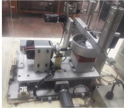
Fig.3 pin-on-disk TE 97 multi-Axis tribometer wear test
